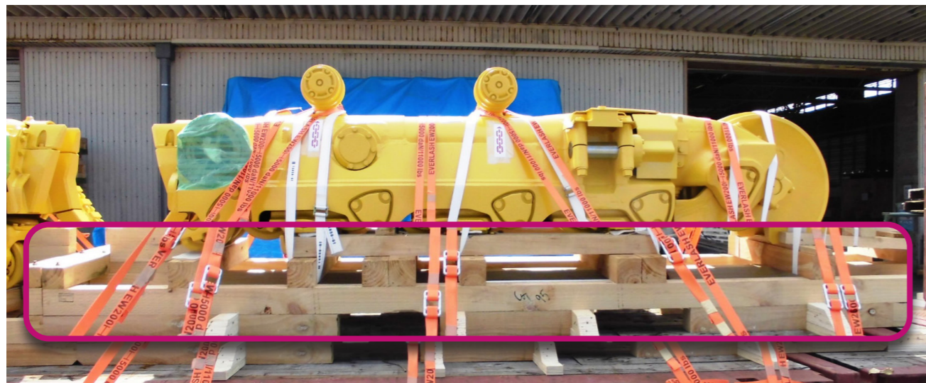
Place thick timber dunnage beneath the cargo to spread the floorboard weight concentration
