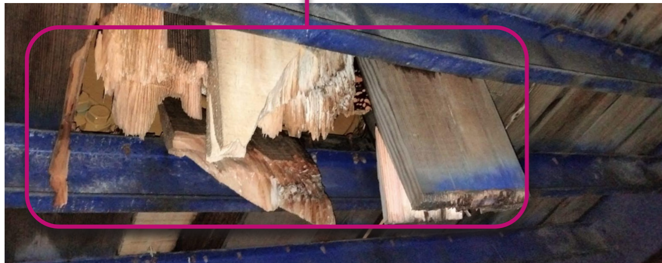
Floorboard damage resulted from exceeding the weight concentration limit
